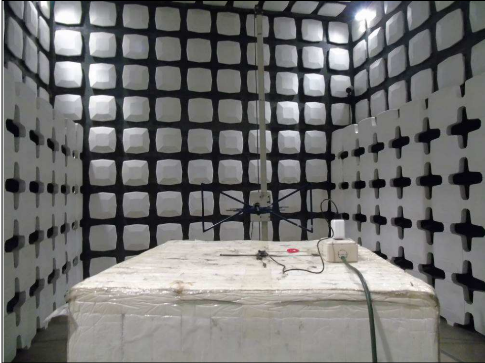
SPURIOUS EMISSION TEST BELOW 1GHz
